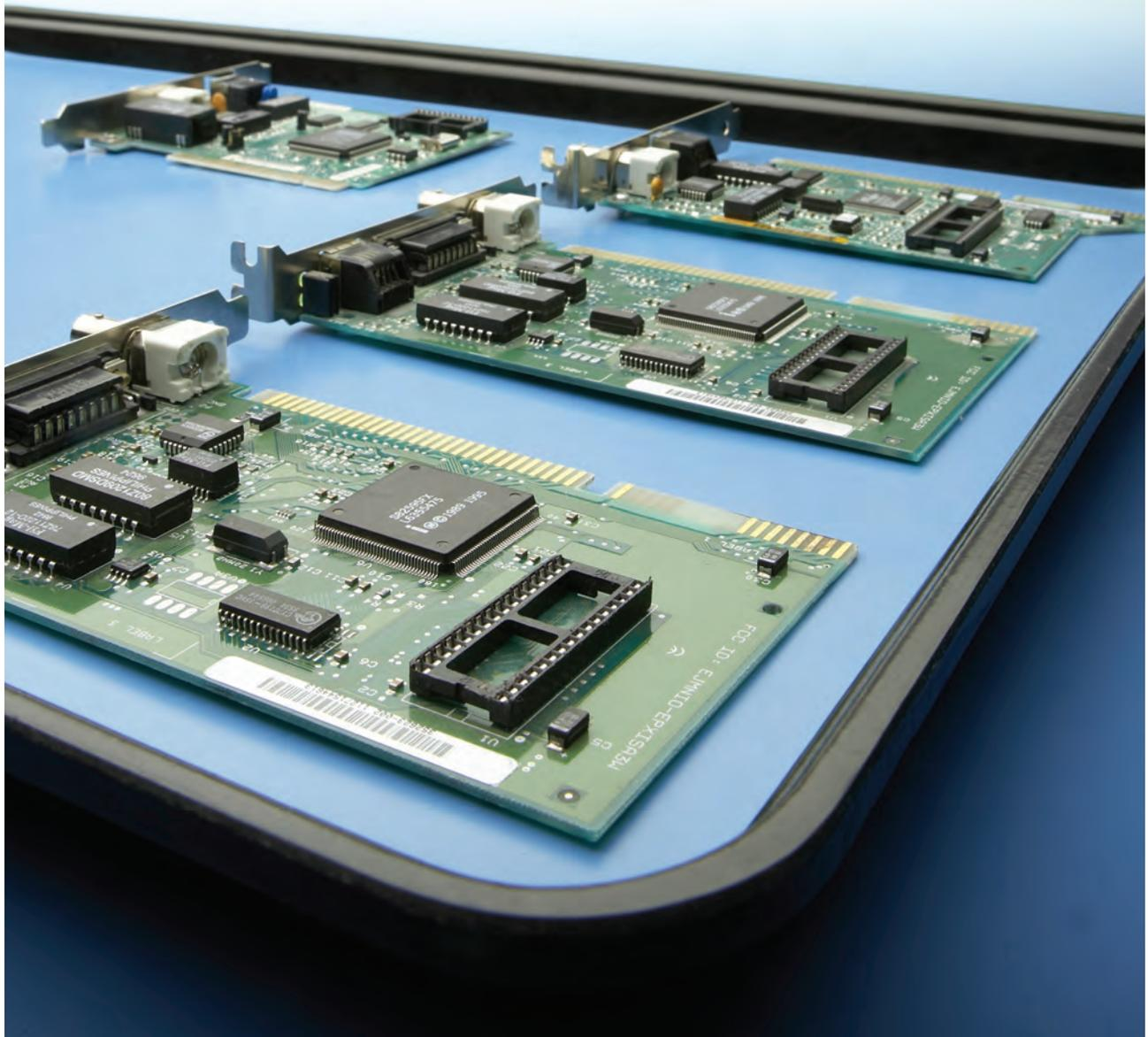
MFG Tray ESD-safe conductive products have a surface resistivity of  $<10^5$  to  $10^6$  ohms. Static dissipative products have surface resistivity between  $10^5$  to  $10^{11}$  ohms. MFG Tray Fibrestat products meet or exceed ANSI/ESD S20.20 standard for ESD protection.
