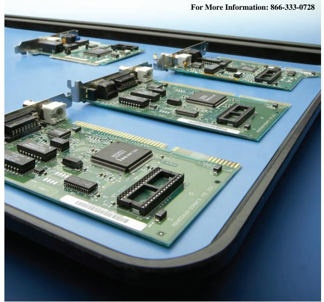
MFG Tray ESD-safe conductive products have a surface resistivity of <10<sup>5</sup> to 10<sup>6</sup> ohms. Static dissipative products have surface resistivity between 10<sup>5</sup> to 10<sup>11</sup> ohms. MFG Tray Fibrestat products meet or exceed ANSI/ESD S20.20 standard for ESD protection.
