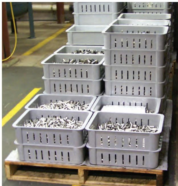
**Kinder than metal.** Composite containers are easier on end products than metal baskets and eliminate the damage or hazard posed by broken wire baskets.
