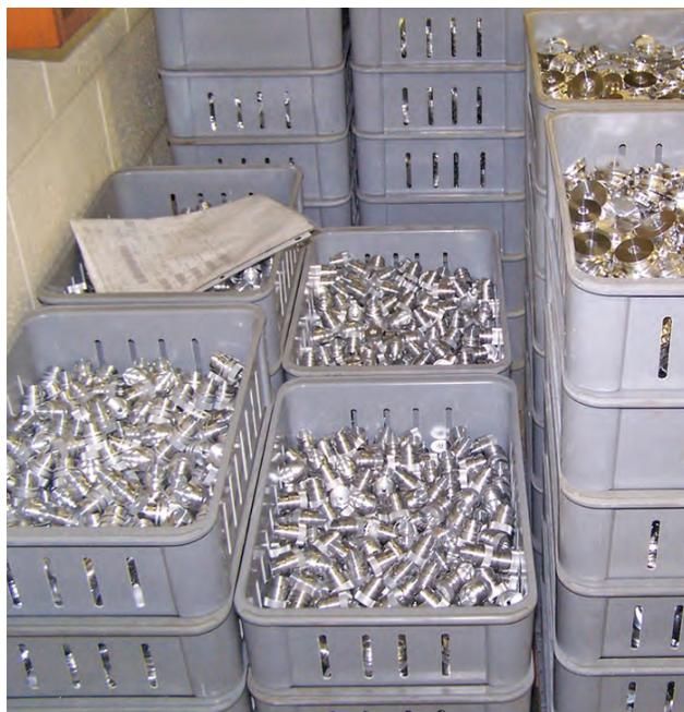
**More efficient material handling and storage.** MFG Tray wash boxes offer the versatility to be used for cleaning, inventory and storage of small parts, and often eliminate the need for dumping product into special containers for the washing process.
