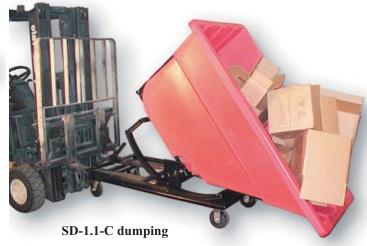
Our molded polyethylene Self-Dumping Hoppers are designed to allow safe and easy handling and dumping of heavy loads. Bins dump up to 40 degrees below horizontal with a simple pull of the handle. Made to work with a forklift, but optional 6" heavy-duty casters allow for easy manual manueverability. Please note: bottom frame should always be secured to the fork lift prior to dumping.
