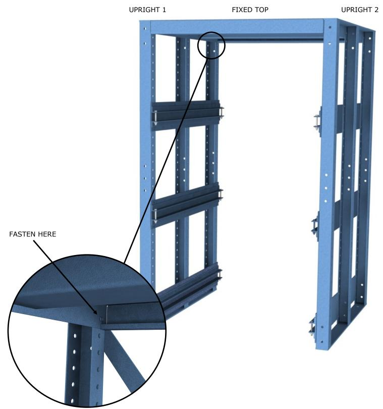
3. Bolt cross bracing to rear of glideout. See view below for proper placement.
