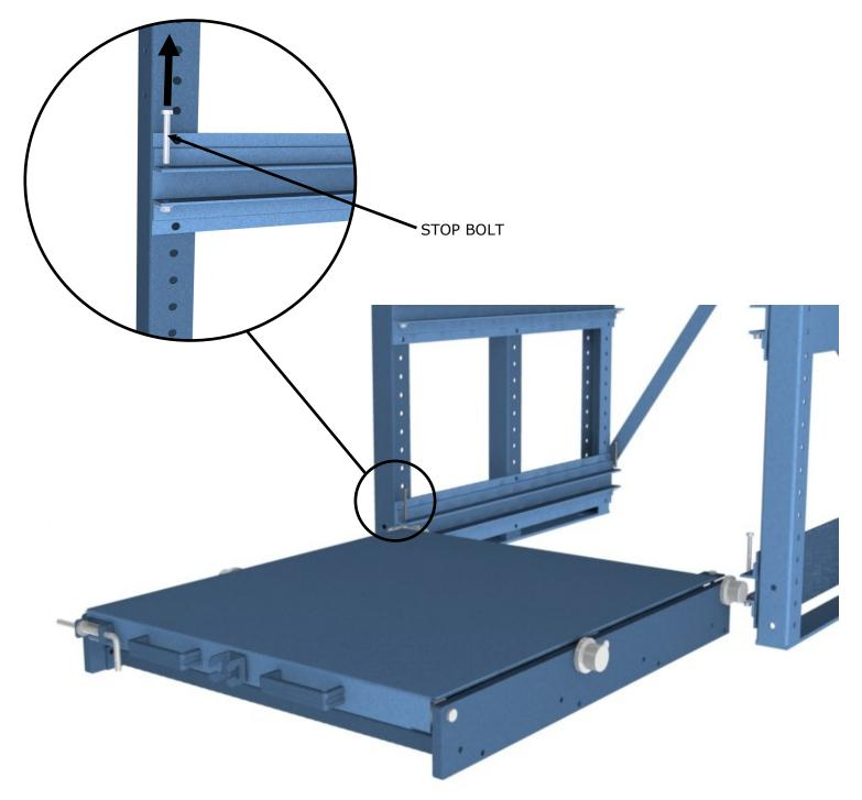
6. Install shelves by inserting cam followers into rail plates, which are bolted to the upright. Once both front and rear cam followers are inserted, push shelf all the way in.
