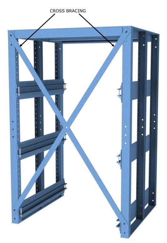
4. Level and anchor glideout frame to floor using the holes provided in the bottom pad of the uprights. Complete a final cross square check to ensure that uprights are square to each other.
