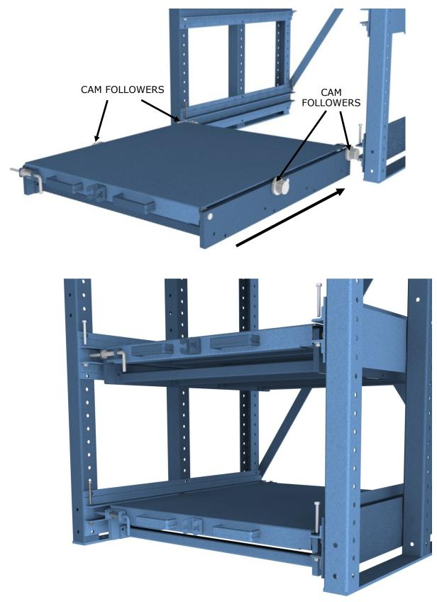
7. Once each shelf is in place reinstall stop bolts into rail plates. Once stop bolts are securely fastened. Pullout each shelf one by one to ensure they function properly. If each shelf pulls out easily installation is completed.
