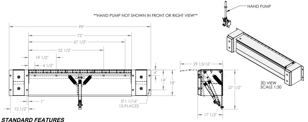
**MODEL NUMBER IS PP-3072 OVERALL WIDTH IS 99" DECK WIDTH IS 72"** OVERALL DEPTH WITH RAMP OUT IS 29 13/16" **BUMPER PROJECTION IS 17 1/2"** UNIFORM CAPACITY IS 30,000 LBS. 5" ABOVE / 5" BELOW SERVICE RANGE HYDRAULIC HAND PUMP OPERATION RECOMMENDED FOR DOCKS AT LEAST 48" HIGH. INCLUDES HAND PUMP, WALL-MOUNT BRACKET, CYLINDER, HYDRAULIC LINES AND OIL. TREADPLATE RAMP & DECK CONSTRUCTION
