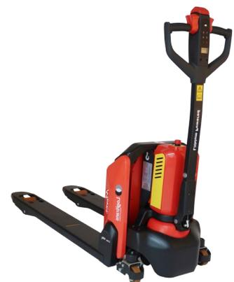
Closed front end in metal for protection
