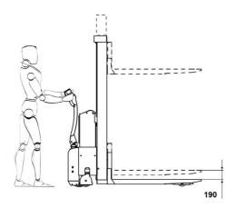
The forks will lift 190 mm before the telescopic mast begins to extend.
