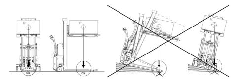
The load centre is never allowed to exceed the center line of the wheels. The driving speed is reduced when lifting the forks above 400 mm. The Logiflex is designed for use on even and level floor. During transport the forks shall be raised as little as possible. Transport with raised forks should be made over the shortest possible distances and at low speed.
