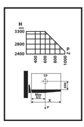
**Specific to Logiflex -** with load limitation at significant lifting heights:
