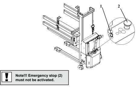
Condition: The upper edge of the forks is lifted between 400 and 900 mm.
