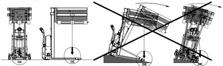
The load centre is never allowed to exceed the centre line of the wheels. The driving speed is reduced when lifting the forks above 400 mm.
