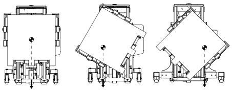
The load centre is not allowed to be placed on the outside of the legs of the stacker, as this will cause a risk of turning over. **NOTE!** Rotation is only allowed to take place, if the Rotator is placed on an equal floor. The load is not allowed to be dislocated during rotation.
