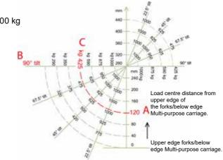
**NOTE!** If the load centre exceeds the allowed distance shown in the load diagram, there is a risk that the Rotator will turn over, when rotating.
