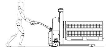
When handling closed pallets - use the Rotator with straddle legs!
