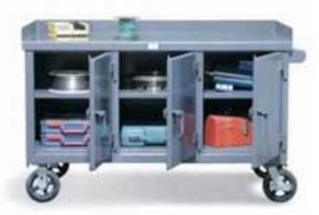
This Mobile work bench has three door openings, 17" wide x 23" high. Three-point lock systems built into each door. It features a 7gauge work surface with a handle for ease in steering, along with two 8" high x 2" deep mold-on rubber swivel casters with brakes and two 8" high x 2" deep mold-on rubber rigid casters.
