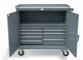
This tool cart has three different sizes of drawers plus an upper compartment for longer tools. The 7-gauge work surface is sturdy enough for most jobs. This cabinet comes equipped with 6" x 2" mold-on rubber casters with floor lock that offer durability, full floor protection and are easyrolling.
